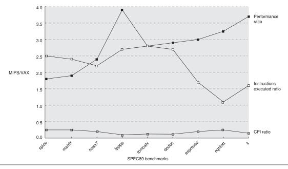
**Figure K.1** Ratio of MIPS M2000 to VAX 8700 in instructions executed and performance in clock cycles using SPEC89 programs. On average, MIPS executes a little over twice as many instructions as the VAX, but the CPI for the VAX is almost six times the MIPS CPI, yielding almost a threefold performance advantage. (Based on data from Bhandarkar and Clark [1991].)
